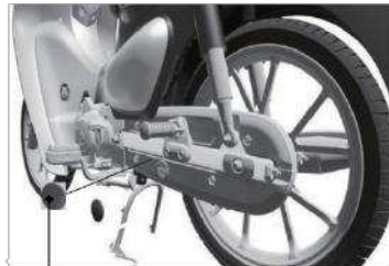
Inspection hole cap
